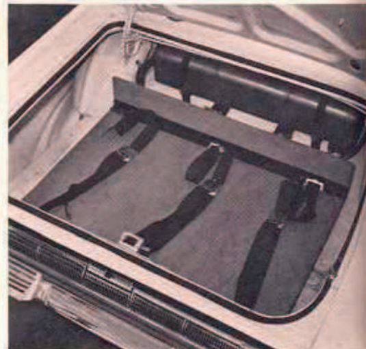
RIGHT—Rear compartment has plywood platform with slide-buckle straps to prevent shovel, jacks, brush knives and towing gear from ricocheting around.
