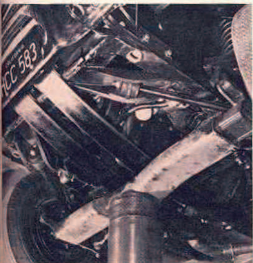
ABOVE — Longitudinal pair of wide, spring steel skids protect oil pan sump from high-centered roads that will be encountered. Suspension is heavy-duty.
