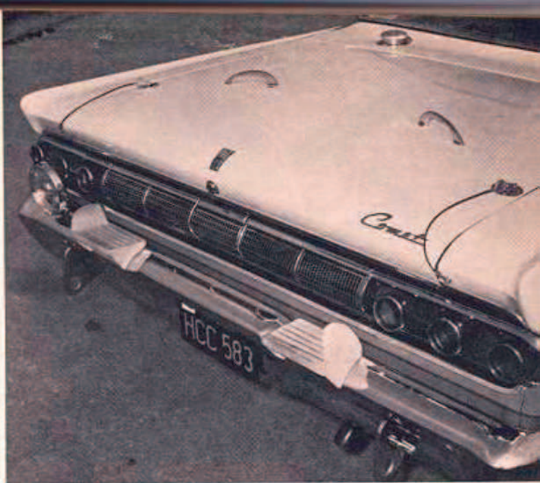
ABOVE LEFT—Standard 20-gallon fuel tank in floor of luggage compartment is supplemented by a 22-gallon reserve over rear axle. Transfer valves permit tank selection. ABOVE RIGHT—A pair of steps on rear bumper plus handles on deck lid provide secure spot for co-driver when extra traction is needed on rear wheels. Note large back-up light, tow eyes in bumper, large diameter gas fill neck. LEFT—Comet bucket seats are retained but catch-all tray replaces console. Speed pilot is mounted over the tunnel. Light switches fill dash center.
